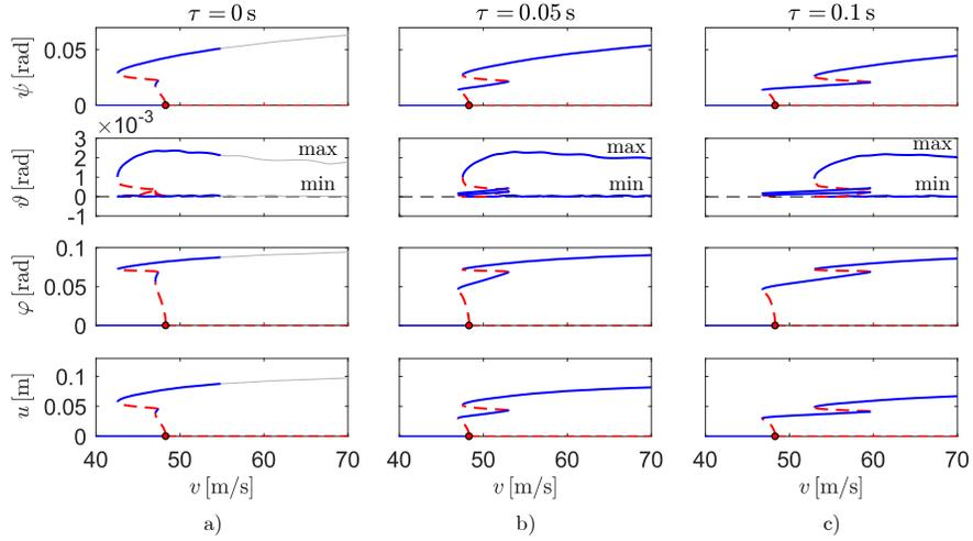
**Fig. 4.** Bifurcation diagrams with respect to the towing speed  $v$  for fixed control gain ( $D = 5000$  Ns) and for different feedback delays: a)  $\tau = 0$ , b)  $\tau = 0.05$  s, c)  $\tau = 0.1$  s
