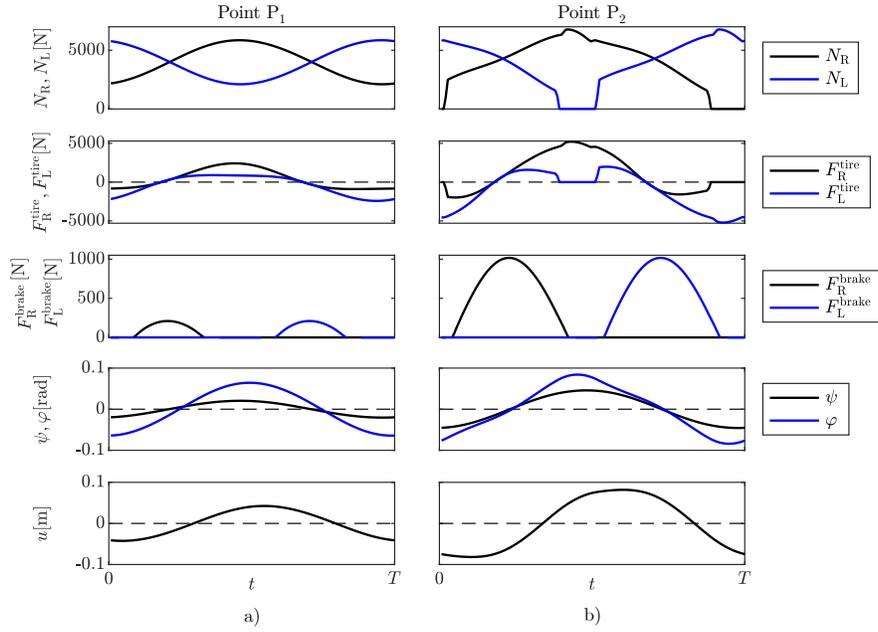
**Fig. 3.** Numerically determined time histories of the normal loads, the tire forces, the braking forces and the generalized coordinates  $\psi$ ,  $\varphi$ , and  $u$ , for control gain  $D = 5000$  Ns and feedback delay  $\tau = 0$ . Panels refer to the points marked in Fig. 2(b).
